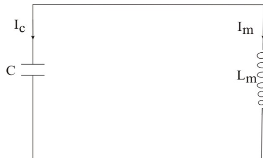
Fig. 1: Highly simplified induction generator equivalent circuit.
