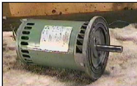
Typical waterpump motor
